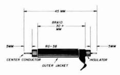
fig. 3. Dimensions for the section RG-58 of coaxial cable used as the primary of the transformer.
